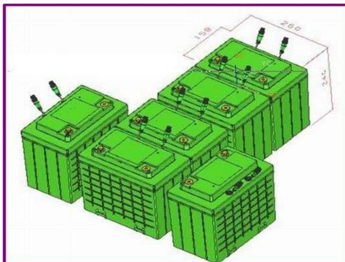
Example of Mono-block style LiFePO4 EV-Battery
