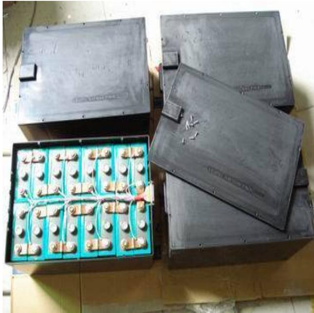
24V LiFePO4 EV-Battery in an 8-Cell Steel Battery-Tray
