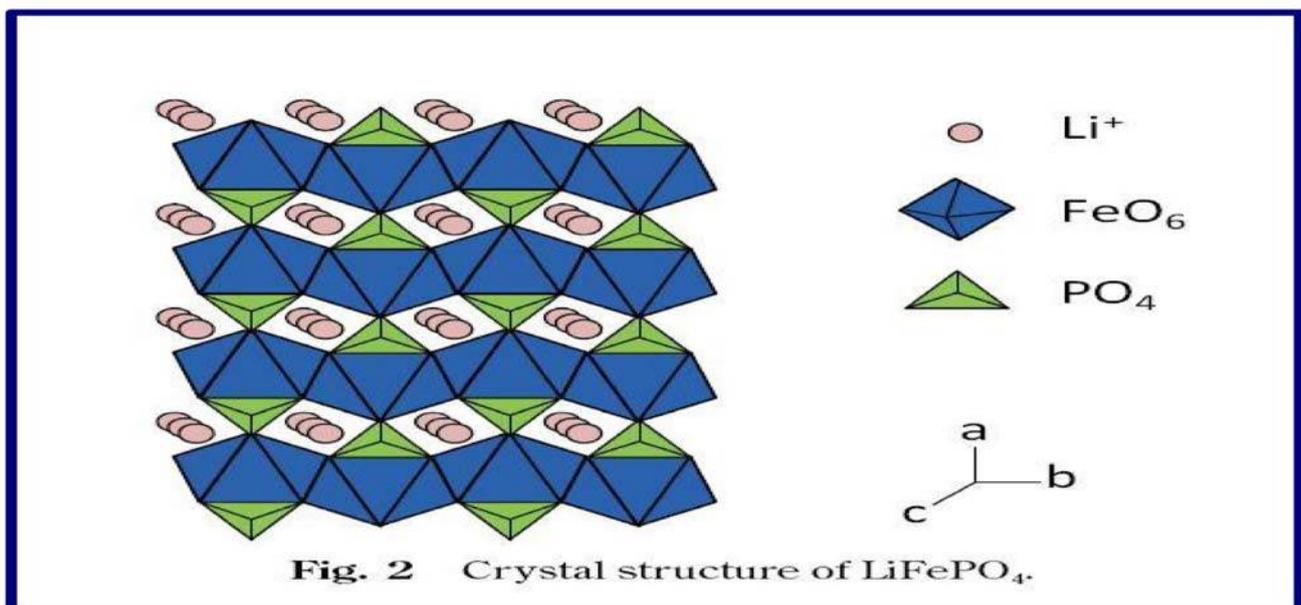
Oxygen atoms show slightly distorted hexagonal close packed arrangement.  $\text{FeO}_6$  is a corner shared octahedron and  $\text{PO}_4$  is an edge-shared tetrahedron, and they form the zigzag skeleton by sharing oxygen and Li ions located in the octahedral channels.
