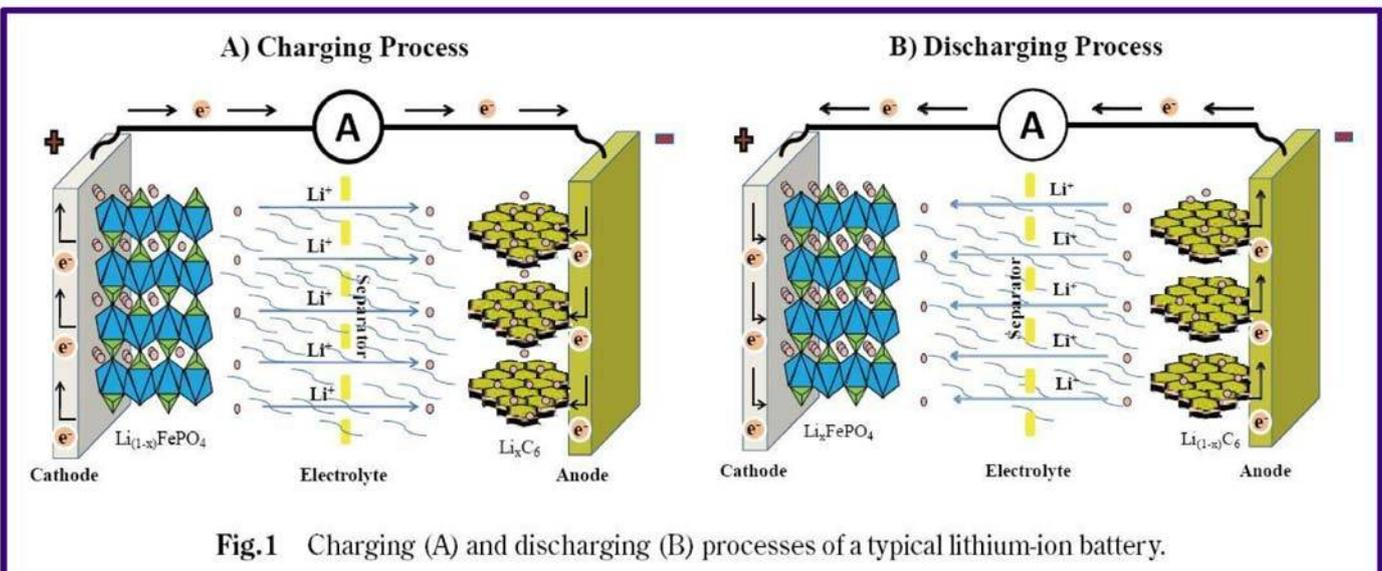
When the battery is charged, lithium ions de-intercalate from the cathode and intercalate into the anode through the electrolyte; while on the discharging process, lithium ions de-intercalate from the anode and intercalate into the cathode.
